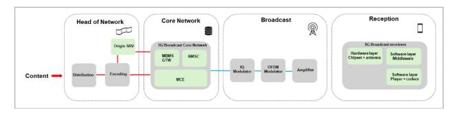
The 5G Broadcast will rely on a core network technical setup to process the broadcast signal and render it in the player, relying on the middleware of mobile terminals.
